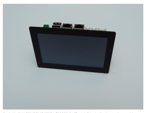
Eval-Kit EVK STM32MP157 DL (50099 045) with 5 inch display and capacitive multitouch. The baseboard is mounted on the backside of the display.
