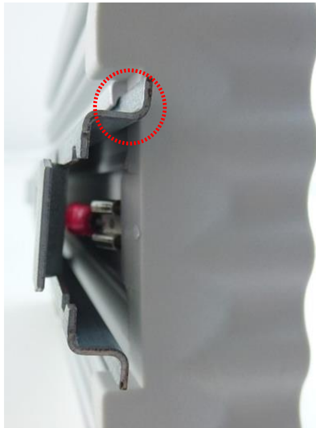
Figure 17: Housing mounted on the DIN rail
