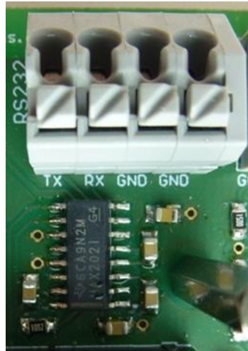
Figure 76: Terminal block connectors - serial interfaces
