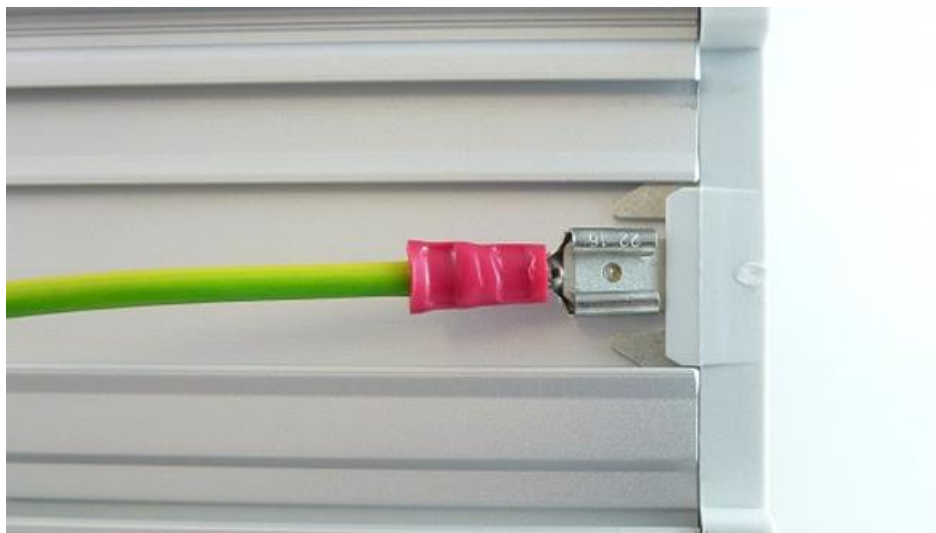
Figure 16: DIN rail housing with grounding connection (PE)
