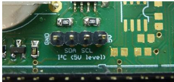
Figure 43: Pin header - I 2 C on 5V level
