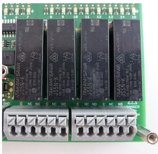
Figure 63: Terminal connection block – relay
