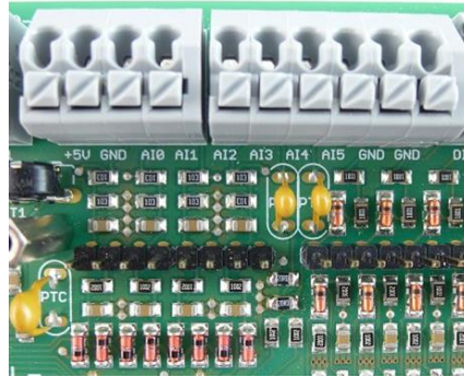
Figure 70: Terminal block - analog inputs
