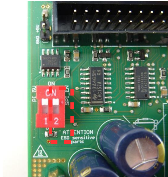
Figure 28: Switch – “SPI_EN”
