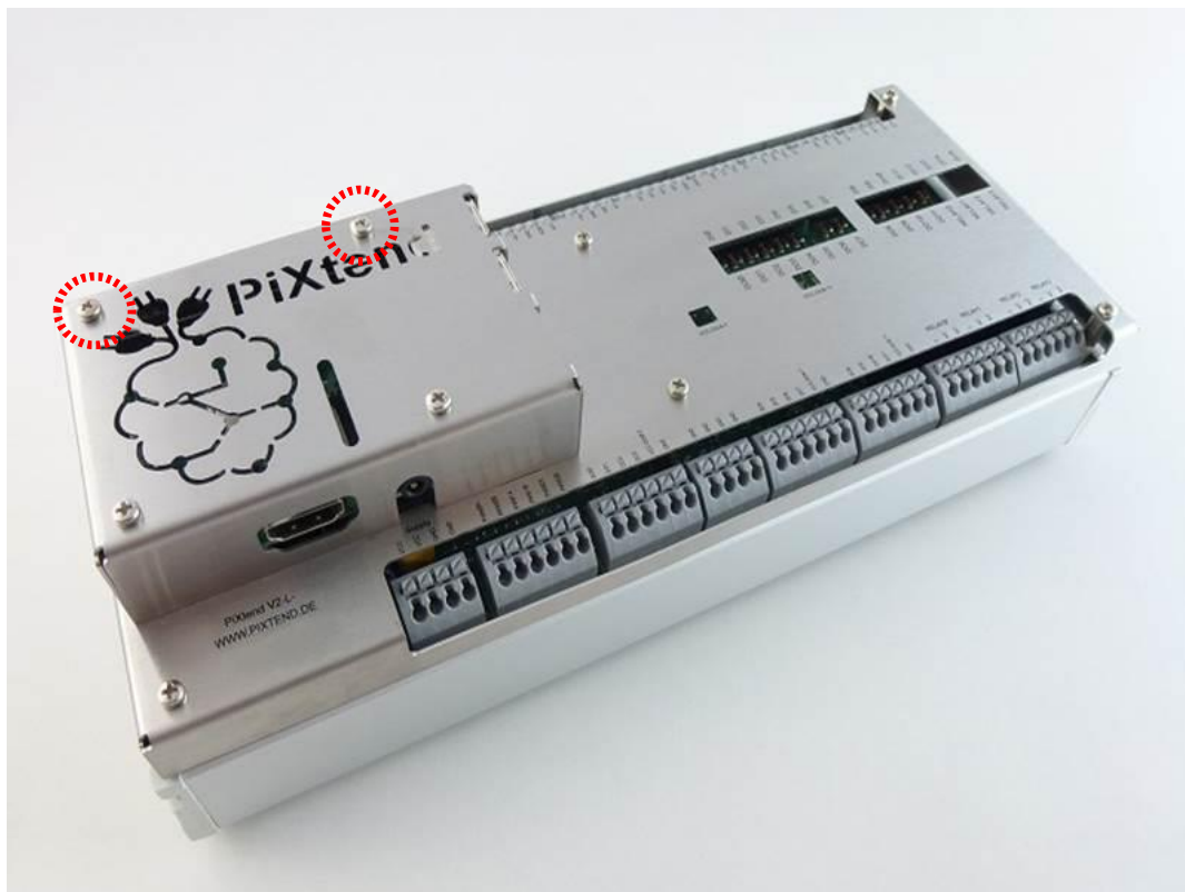
Figure 26: Completely assembled stainless-steel cover
