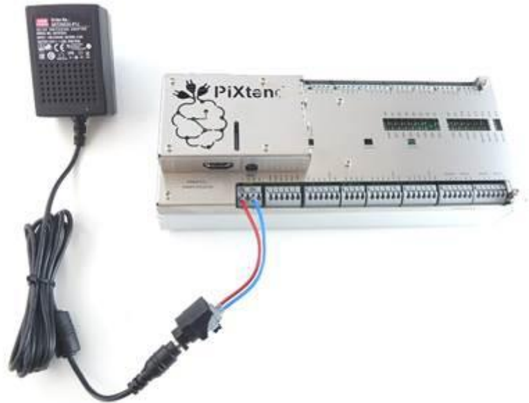
Figure 40: Power supply connected to the PiXtend V2 -L-
