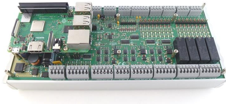
Figure 14: Assembled DIN rail housing
