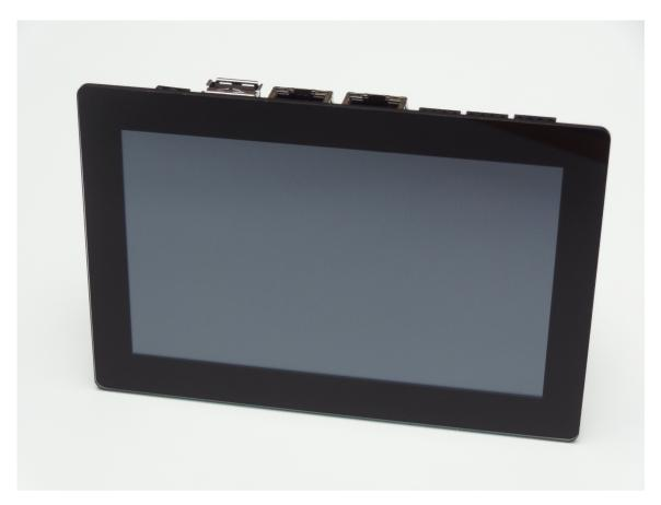
Demo-Kit with 5 inch display and capacitive multitouch. The baseboard is mounted on the backside of the display.
