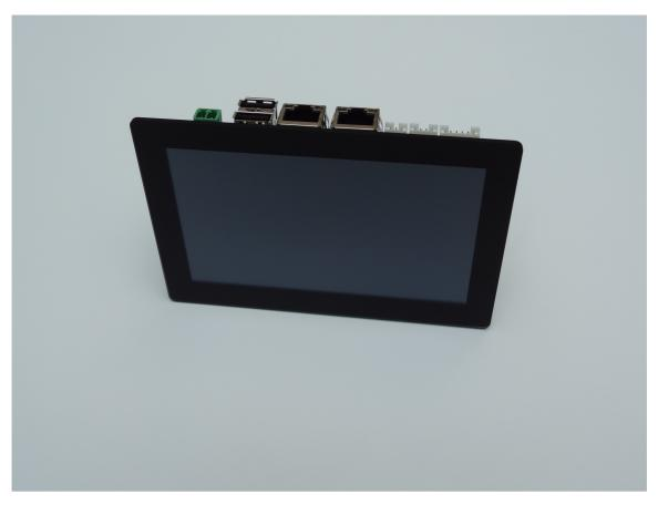
Demo-Kit DK STM32 SOM MP157 (50099044 rev00) with 5 inch display and capacitive multitouch. The baseboard is mounted on the backside of the display.
